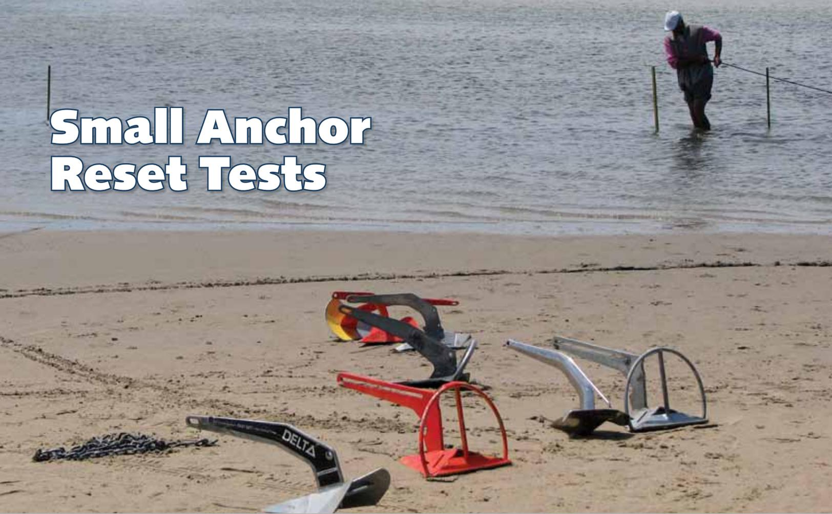
The most controlled aspect of the anchor testing took place on a sand and clay bottom near Sydney, Australia. The comparison featured traditional designs, and a variety of newer “convex” fluke designs (foreground) and “concave” designs (background).
