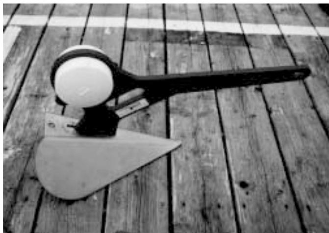
**Left:** The circular plastic float material clamped in the back of the shank is supposed to assure that the Hydro-Dyne anchor settles upright on the bottom, which then engages the bottom with the stainless steel plow. Practical Sailor could not get the anchor, when dropped in the water, to assume the proper position. This anchor retails for \$165.
