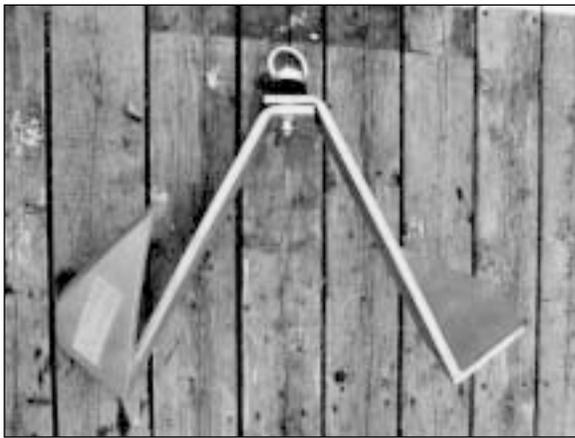
**Above:** New in the US, the unusual Seagrip was invented by a pair of Swedish fishermen. Acting somewhat like a propeller, the Seagrip is supposed to screw itself into the bottom (we assume greater loads than we developed would be required for this action to occur). In sand, it set in less than 3', but developed only 240 lbs. of holding power. The Seagrip (\$325) is shown folded in the smaller photo.
